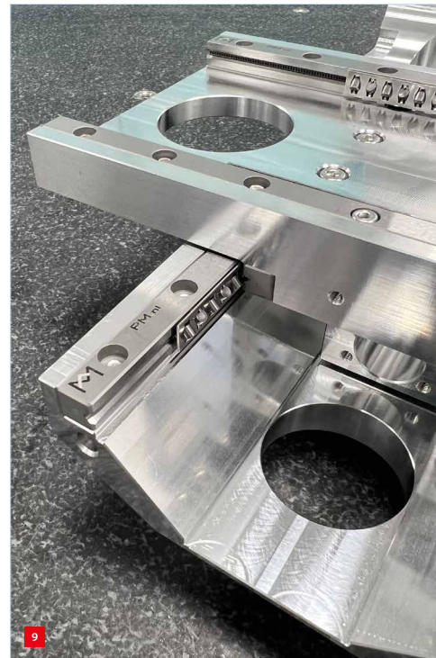
Example of an overrunning cage.
